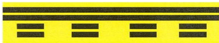
RSA/OFZ BOUNDARY SIGN
