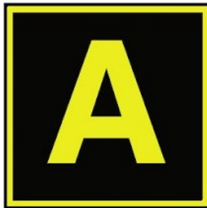
TAXIWAY LOCATION SIGN
